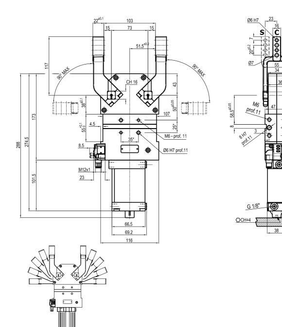
Bore<br/>ØClamping<br/>momentWeight ( clamping<br/>arms not included)40 mm55 Nm2.7 Kg
