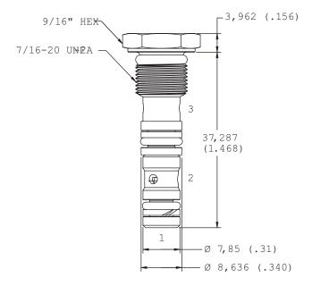
Note: Torque cartridge in aluminum or steel housing 8.1-13.6 Nm (6-10 ft lbs).
