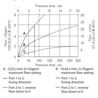
C - 3,8 L/min (1 USgpm) maximum flow setting
