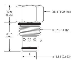
Torque cartridge in housing: A - 47-54 Nm (35-40 ft lbs) S - 68-75 Nm (50-55 ft lbs)
